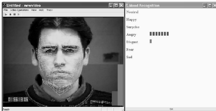
Fig. 1: A snap shot of our realtime facial expression recognition system. On the left side is a wireframe model overlaid on a face being tracked. On the right side the correct expression, Angry, is detected.
