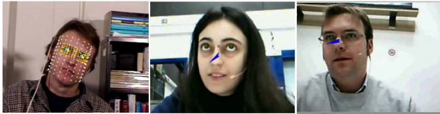
Figure 1. (a) View-normalized eye-center estimation using CHM and eye-center locator. (b),(c) are examples where direction of social visual attention is different from head-pose direction. Blue triangular-normal denotes head-pose while green circles represent eye locations.
